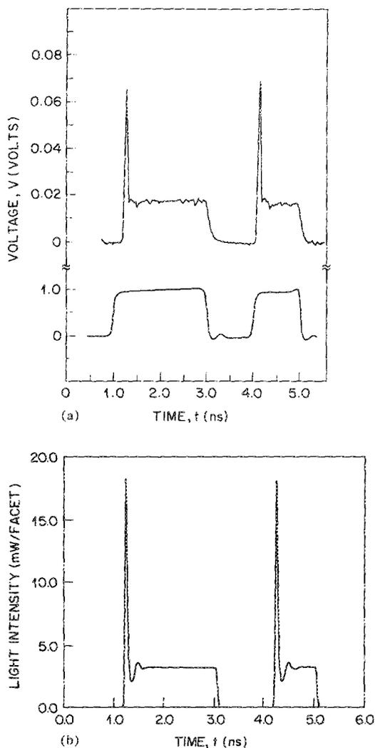
FIG. 3. (a) Oscilloscope trace of  $p-i-n$  receiver output (upper curve) to a ...011010...  $1 \text{ Gbit s}^{-1}$  NRZ data stream  $V_S$  (lower curve) applied to saturable absorber  $S$ . Data taken with  $I_G = 70 \text{ mA}$ . (b) Calculated response of the multielectrode laser to a...011010...  $1 \text{ Gbit s}^{-1}$  NRZ data stream applied to saturable absorber  $S$ .
