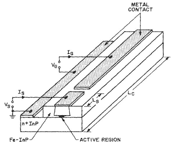
FIG. 1. Schematic sketch of a BH GRINSCH four quantum well laser diode with a cavity length  $L_C$  and an intracavity absorber of length  $L_S$ . The current into the long gain section is  $I_G$ , the absorber voltage and current are  $V_S$  and  $I_S$ , respectively.
