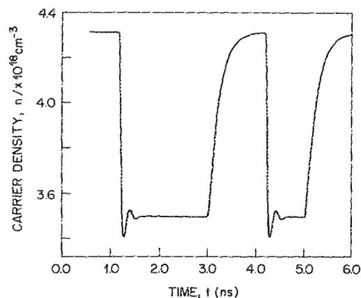
FIG. 4. Calculated variation in carrier density during application of a  $1 \text{ Gbit s}^{-1}$  NRZ data stream to saturable absorber  $S$ .
