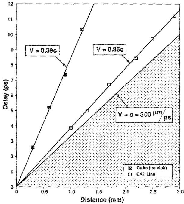
FIG. 2. Plot of delay (as measured by midpoint of linear fit to rise time) vs propagation distance. Velocity  $V$  is found from a linear fit to the data. Shaded area is bordered by  $V = c$ .
