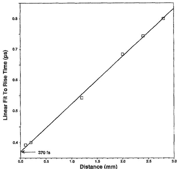
FIG. 4. Plot of rise time (as measured by midpoint of linear fit to rise time) vs propagation distance. The zero distance intercept gives a system response rise time of 370 fs. Measured rise time after 2.8 mm of propagation is 0.8 ps.
