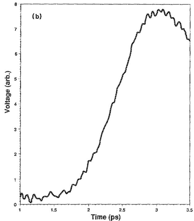
FIG. 3. (a) Measured signal on CAT line after 75  $\mu\text{m}$  of propagation. (b) Measured signal on CAT line after 2.8 mm of propagation showing rise time of 0.8 ps.
