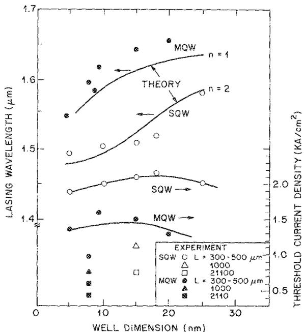
FIG. 3. Laser wavelength and threshold current density plotted as a function of the well thickness. The calculated lines represent the  $n = 1$  and  $n = 2$  confined particle state of the entire quantum well GRIN structure.
