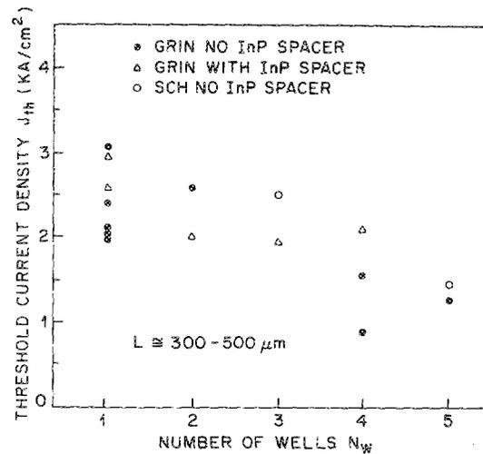
FIG. 2. Broad-area threshold current density plotted as a function of the number of quantum wells. No significant increase in the threshold current density is observed for the single quantum well.
