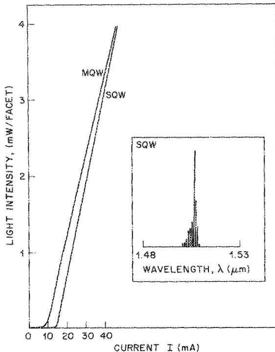
FIG. 4. Light-current characteristics and lasing spectrum of a buried-heterostructure laser based on a single and multiple quantum well GRIN SCH structure.
