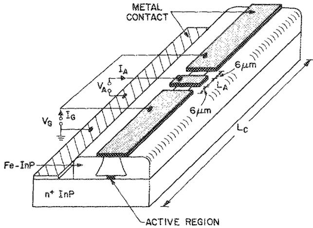
FIG. 3. Sketch of the BH GRINSCH SQW laser diode with a cavity length  $L_C$  and an absorber length  $L_A$ . The gain current  $I_G$  into the large segments, the absorber voltage  $V_A$ , and absorber current  $I_A$  at the small segment are indicated.
