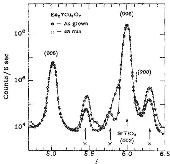
FIG. 4. Scan along [001] for the as-grown film (●) and after 45 min of milling (○). The peaks marked "x" are SrTiO<sub>3</sub> impurities also seen in the bare substrate. Note that the weak (200) feature, identified as an *a*-axis component of the film, disappears after the first stage of milling.
