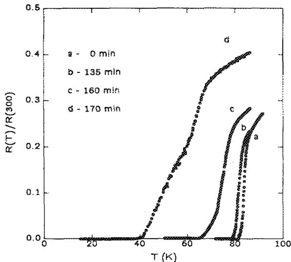
FIG. 2. Plot of the resistive transitions, normalized to the respective room-temperature resistances, for four different stages of milling identified in the legend and in Fig. 1. The temperature coefficient of resistance is positive up to room temperature.
