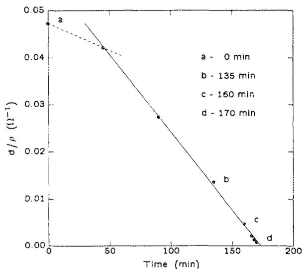
FIG. 1. Plot of the room-temperature sheet conductance vs milling time. The labeled points, with milling times identified in the legend, correspond to the resistive transitions in Fig. 2. The dashed line corresponds to the slow removal of *a*-axis-oriented material initially at the surface and the solid line indicates a uniform removal of *c*-axis material.
