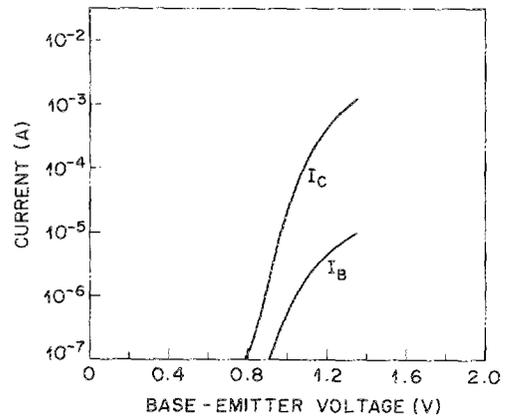
FIG. 3. Transfer characteristics of the collector current  $I_C$  and base current  $I_B$  as a function of the base-emitter voltage for transistor with emitter size of  $0.6 \times 7 \mu\text{m}^2$ .
