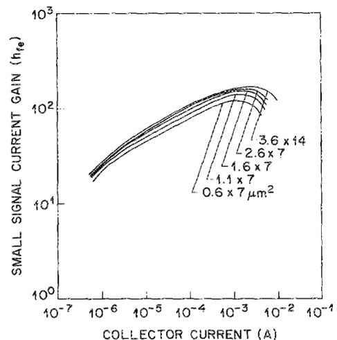
FIG. 4. Common-emitter gain as a function of collector current for different emitter dimensions  $0.6 \times 7$ ,  $1.1 \times 7$ ,  $1.6 \times 7$ ,  $2.6 \times 7$ ,  $3.6 \times 14 \mu\text{m}^2$ .
