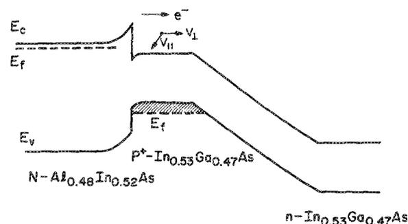
FIG. 1. Energy-band diagram for the  $\text{AlInAs}/\text{InGaAs}$  heterostructure bipolar transistor.
