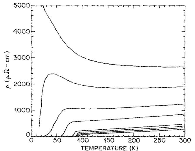
FIG. 2. Series of  $R$  vs  $T$  plots for a high quality  $\text{YBa}_2\text{Cu}_3\text{O}_{7-x}$  film (No. 2 from Fig. 1) showing the transition from superconducting to insulating behavior as a function of 1 MeV  $\text{Ne}^+$  fluence. For increasing resistivity, the fluences are (from the bottom curve up): undamaged, 1.0, 2.5, 4.0, 10.0, 15.0, 20.0, and  $22.0 \times 10^{13}$ /cm<sup>2</sup>.
