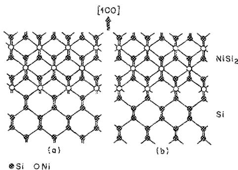
FIG. 3.  $\text{NiSi}_2/\text{Si}(100)$  interface as viewed in the (a)  $[011]$  and (b)  $[0\bar{1}1]$  projections. A rigid shift displacement of  $a/4\langle 111 \rangle$  is required to join the two sections of interface.
