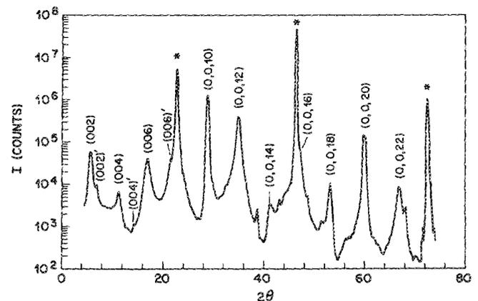
FIG. 3.  $\theta$ - $2\theta$  x-ray diffraction scan for a film of Ca-Sr-Bi-Cu oxide on  $\langle 100 \rangle$   $\text{SrTiO}_3$ , measured with Cu  $K_\alpha$  radiation. The diffraction lines from the 80 K superconducting phase and a related semiconducting phase are designated  $(00l)$  and  $(00l)'$ , respectively. The  $(h00)$  lines from the  $\text{SrTiO}_3$  substrate are indicated with an asterisk.
