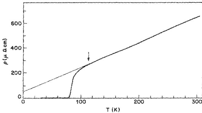
FIG. 1. Temperature dependence of the resistivity (heavy line) for a film of composition  $\text{Ca}_{1.00}\text{Sr}_{1.58}\text{Bi}_{2.35}\text{Cu}_{3.94}\text{O}_x$ , grown on  $\langle 100 \rangle$   $\text{SrTiO}_3$ . A weak, although characteristic break in slope at  $T \sim 115$  K is indicated with an arrow. The fine line shows the projected intercept of the linear portion of  $\rho(T)$  at  $T = 0$ .
