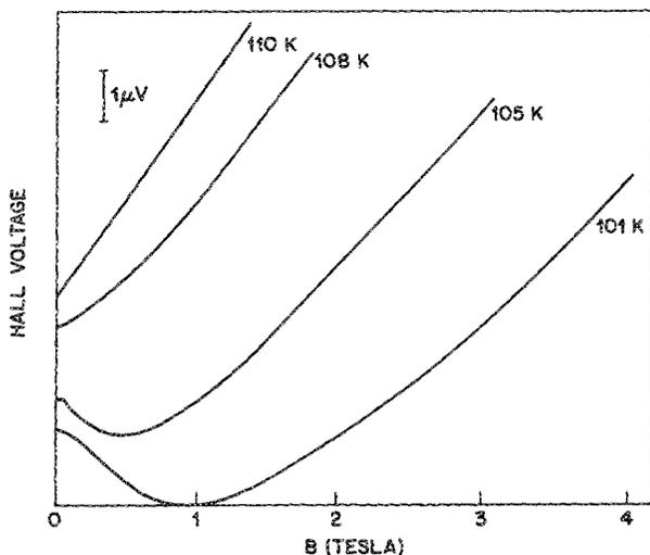
FIG. 2. Hall voltage vs magnetic field  $B$  for the film of Fig. 1, at temperatures near  $T_c$ . The curves have been offset for clarity.
