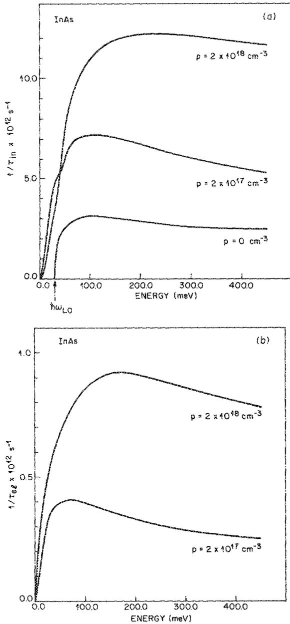
FIG. 3. (a) Total inelastic electron scattering rate as a function of electron energy measured from the conduction-band minimum for different carrier densities in  $p$ -type InAs. (b) Total elastic electron scattering. Parameters used in calculations were  $m_1 = 0.41m_0$ ,  $m_2 = 0.025m_0$ ,  $m_3 = 0.021m_0$ ,  $\epsilon_\infty = 11.8$ ,  $\hbar\omega_{LO} = 30.2$  meV, and  $\hbar\omega_{TO} = 27.1$  meV.
