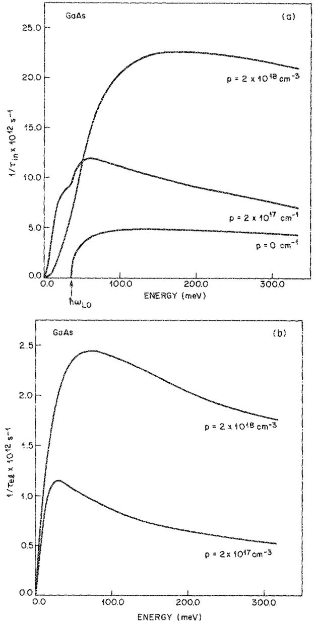
FIG. 2. (a) Total inelastic electron scattering rate  $1/\tau_{\text{in}}$  as a function of electron energy measured from the conduction-band minimum for different carrier densities in  $p$ -type GaAs. (b) Total elastic electron scattering. Parameters used in calculations were  $m_1 = 0.5m_0$ ,  $m_2 = 0.082m_0$ ,  $m_3 = 0.07m_0$ ,  $\epsilon_\infty = 10.91$ ,  $\hbar\omega_{\text{LO}} = 36.5 \text{ meV}$ , and  $\hbar\omega_{\text{TO}} = 33.8 \text{ meV}$ .
