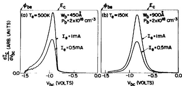
FIG. 5. Hot-electron spectra, measured at 4.2 K, for a double heterojunction bipolar transistor having (a) a 900-Å base width and (b) a 450-Å base width. The inferred electron temperature is indicated in the figures.
