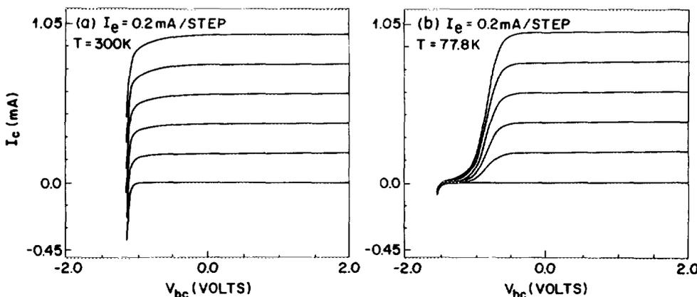
FIG. 4. Common base characteristics of the double heterojunction bipolar transistor having a 900-Å base region measured at (a) 300 K and (b) 77.8 K.
