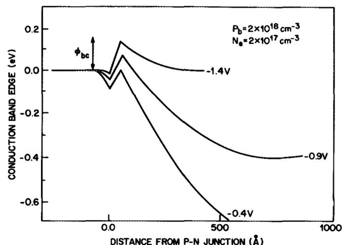
FIG. 2. Calculated variation of the base/collector conduction-band edge with distance at indicated values of forward bias.
