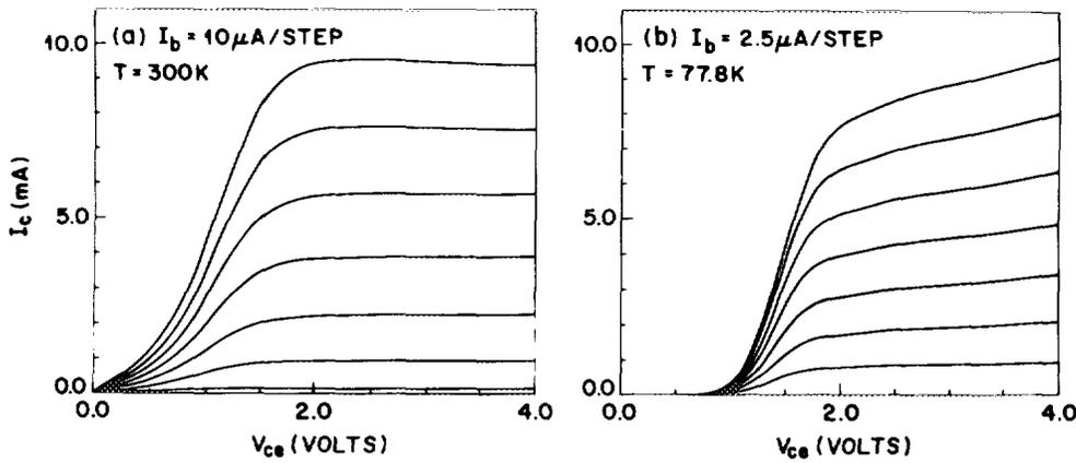
FIG. 3. Common emitter characteristics of the double heterojunction bipolar transistor having a 900-Å transit region measured at (a) 300 K and (b) 77.8 K. The emitter mesa diameter is 100 μm.
