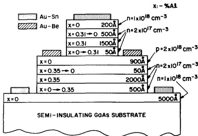
FIG. 1. Schematic diagram of the layer structure comprising the double heterojunction bipolar transistor having the 900-Å base region. The fraction of Al present in each layer is given by *x*.
