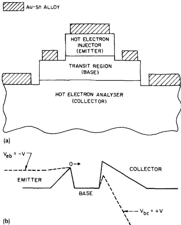
FIG. 1. Schematic diagram of the MBE grown GaAs epilayers comprising the two level mesa structure are shown in (a) together with a schematic of the conduction-band edge of the hot-electron injector (emitter), transit region (base), and hot-electron analyzer (collector) in (b). The broken lines indicate the conduction-band edge of the structure when biased.
