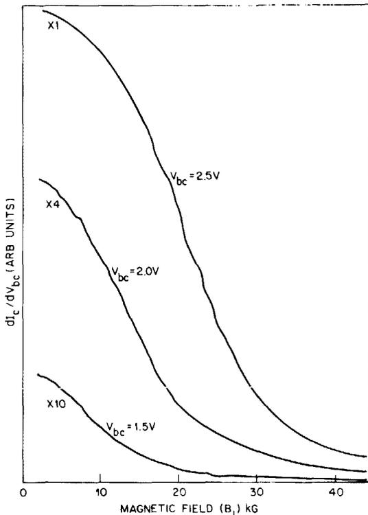
FIG. 3. Variation of spectral intensity with applied magnetic field for three indicated hot-electron analyzer (collector) biases.
