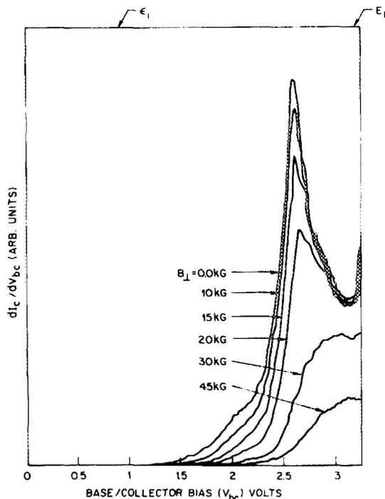
FIG. 2. Magnetic field dependence of a hot-electron spectrum when a magnetic field is applied perpendicular to the direction of current flow at the hot-electron injector (emitter). The injection energy  $\epsilon_i$  and the position of the Fermi energy  $E_F$  are indicated for this particular sample having a transit region width of  $1200 \text{ \AA}$ .
