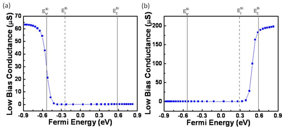
FIG. 3. Low bias conductance plotted as a function of graphene Fermi energy for (a) graphene-Si (*p*-type) and (b) graphene-Si (*n*-type) devices. The right and left solid vertical lines represent the conduction and valence bands of silicon, and the middle dashed line represents the Fermi energy of silicon.
