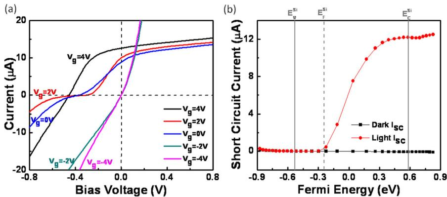
FIG. 4. (a) Graphene-silicon  $I$ - $V_{\text{bias}}$  characteristics taken under illumination at different gate voltages. (b) Short circuit current ( $I_{\text{sc}}$ ) with and without illumination plotted as a function of graphene Fermi energy.
