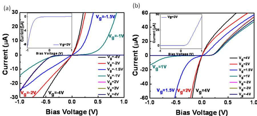
FIG. 2.  $I$ - $V_{\text{bias}}$  characteristics taken at different gate voltages ( $V_g$ ) of (a) graphene-Si ( $p$ -type) and (b) graphene-Si ( $n$ -type) devices. The inset figures show the  $I$ - $V$  characteristics at  $V_g = 0$  V.
