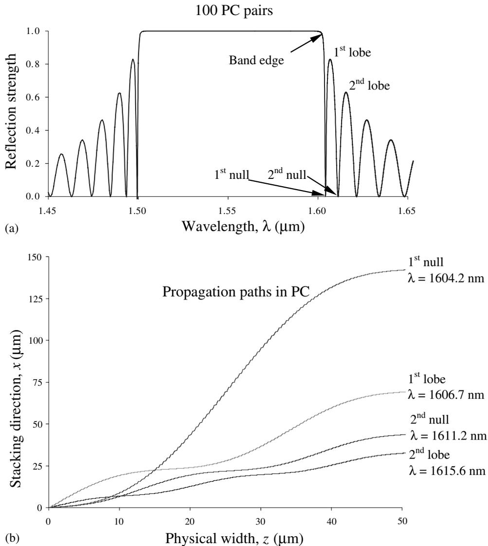
Fig. 2. (a) Reflection spectrum of 100 pairs of periodic dielectric structure, with  $n_1 = 1.5$ ,  $n_2 = 1.65$  and  $d_1 = 0.258 \mu\text{m}$ ,  $d_2 = 0.235 \mu\text{m}$ . The length of one period is  $A = 0.493 \mu\text{m}$ . (b) Average propagation path for beams incident with 15° angle at different wavelengths. The dispersion angle is the largest for the first null in the reflection spectrum.
