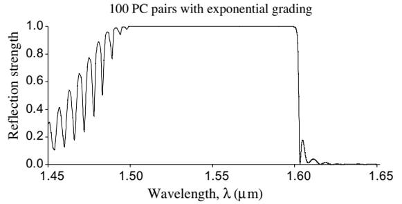
Fig. 7. Reflection spectrum of 100 pairs of PC and 50 pairs of exponential grading pairs ( $m = 5$ ) at each side of the PC. The refractive index for each material is  $n_1 = 1.5$ ,  $n_2 = 1.65$  and the thickness of each material layer is  $d_1 = 0.258 \mu\text{m}$ ,  $d_2 = 0.235 \mu\text{m}$  respectively. The total length of one period is  $\Lambda = 0.493 \mu\text{m}$ . The strong reflection at the first peak is significantly reduced, but the dispersion angle is also decreased.
