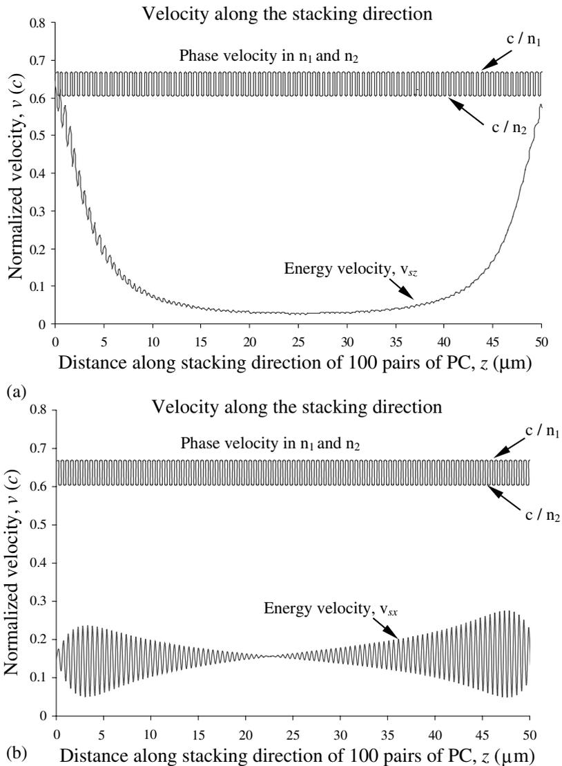
Fig. 3. (a) Energy velocity of the first null in Fig. 2 along the stacking direction in the same dielectric structure as Fig. 2. (b) Energy velocity of the first null in Fig. 2 perpendicular to the stacking direction in the dielectric structure.
