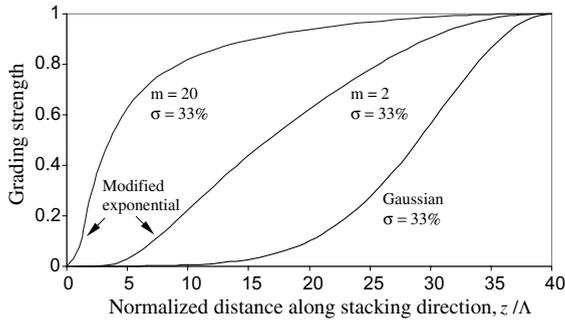
Fig. 6. (a) Grading profile of the modified exponential function for sharpness factor  $m = 20$  and  $m = 2$ ,  $\sigma = 33\%$ . When  $m$  is larger, the initial slope of increase is larger. (b) Grading profile of the Gaussian function with  $\sigma = 33\%$ . The initial grading sharpness is very small compared to the modified exponential grading.
