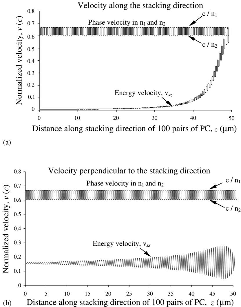
Fig. 4. (a) Energy velocity along the stacking direction in the 100 pairs periodic dielectric structure with  $n_1 = 1.5$ ,  $n_2 = 1.65$  and  $d_1 = 0.258 \mu\text{m}$ ,  $d_2 = 0.235 \mu\text{m}$ . The length of one period is  $\Lambda = 0.493 \mu\text{m}$  and incident angle =  $15^\circ$ . The incident wavelength is near the band-edge. (b) Energy velocity perpendicular to the stacking direction in the dielectric structure at the same wavelength for the same structure.
