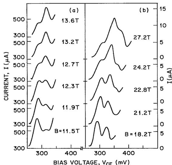
FIG. 4. Portions of  $I_C$ - $V_{CE}$  traces near the anticrossings (a) at  $\omega_C = \frac{1}{2}\omega_{LO}$  for the 30-Å barrier sample and (b) at  $\omega_C = \omega_{LO}$  for the 40-Å barrier sample. Note the different current scales and zero offsets.
