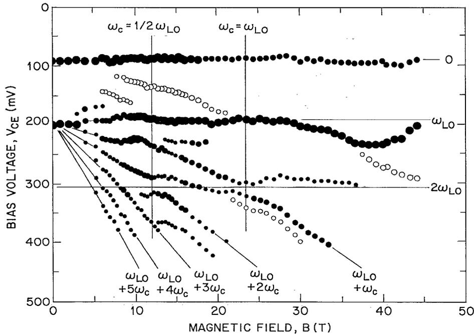
FIG. 2. Resonant tunneling peak positions vs magnetic field. The three circle sizes are proportional to the observed contribution to current (spectral weight). Open circles denote transitions forbidden except in the presence of (e.g., static) disorder. The natural energy and magnetic-field scales are given on the right-hand side and top. Note the anticrossings at the  $2\omega_{LO}$  energy for  $\omega_C = \frac{1}{2}\omega_{LO}$  and  $\omega_C = \omega_{LO}$ .
