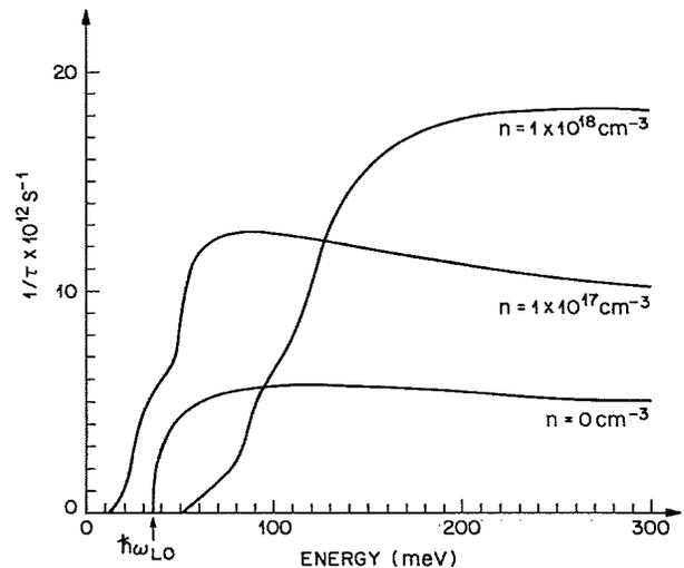
FIG. 2. Total inelastic scattering rate as a function of hot-electron energy measured from the bottom of the conduction band for the indicated carrier densities in GaAs.
