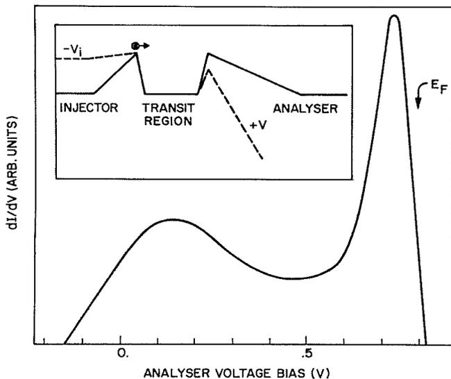
FIG. 1. Hot-electron spectrum for a sample having a 650-Å transit region and  $n = 1 \times 10^{18} \text{ cm}^{-3}$ . The Fermi energy,  $E_F$ , is indicated. Inset: schematic of the conduction-band edge of the hot-electron injector, the transit region, and the hot-electron analyzer. The broken lines indicate the conduction-band edge of the structure when biased with voltage  $-V_i$  at the injector and  $+V$  at the analyzer.
