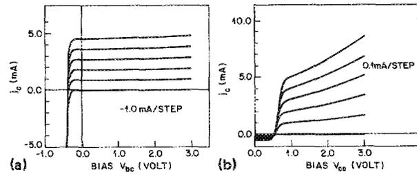
FIG. 2. (a) Room temperature common base current gain characteristics. Curves were taken in steps of  $-0.1 \text{ mA}$  starting with zero emitter injection current. (b) Room temperature common emitter current gain characteristics. Curves were taken in steps of  $0.1 \text{ mA}$  beginning with zero injected base current. Emitter area is  $7.8 \times 10^{-5} \text{ cm}^2$ .
