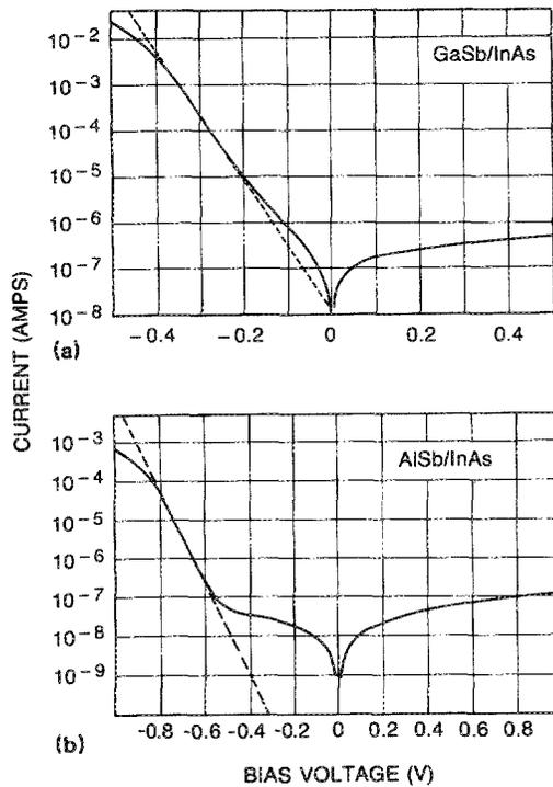
FIG. 1. Current-voltage characteristics of the (a) GaSb/InAs (active area is  $2.0 \times 10^{-4} \text{ cm}^2$ ) and (b) AlSb/InAs (active area is  $7.8 \times 10^{-5} \text{ cm}^2$ ) heterojunctions measured at room temperature.
