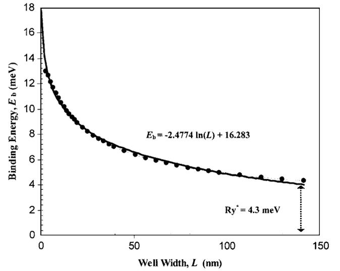
FIG. 2. Exciton binding energy calculated using the tight-binding Hamiltonian as a function of quantum well width for  $\text{Al}_{0.3}\text{Ga}_{0.7}\text{As}/\text{GaAs}$  quantum well structures. The grey line represents a logarithmic fit to data which approximates the function away from the limits of large and small  $L$ .
