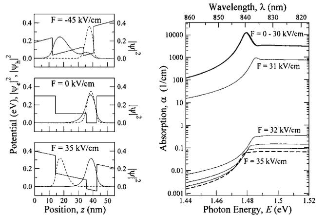
FIG. 4. Broken-symmetry quantum well structure obtained by modifying the structure from Fig. 3 to fit a target functionality: Rapid decrease of the absorption peak with increasing electric field  $F$ , small change in absorption peak energy, and stability with respect to crystal growth inaccuracies. The absorption peak diminishes with the application of either positive or negative electric field. Absorption spectra are shown in increments of 1 kV/cm.
