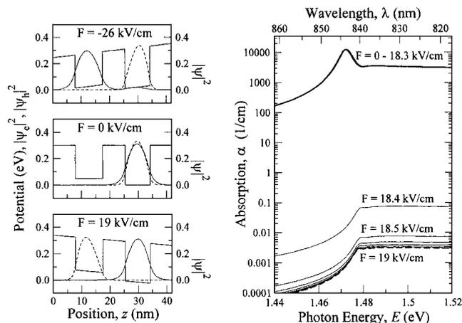
FIG. 6. Asymmetric double quantum well intensity modulator discovered by machine-based exploration without human specification of a target function. Absorption spectra are shown in increments of 0.1 kV/cm.
