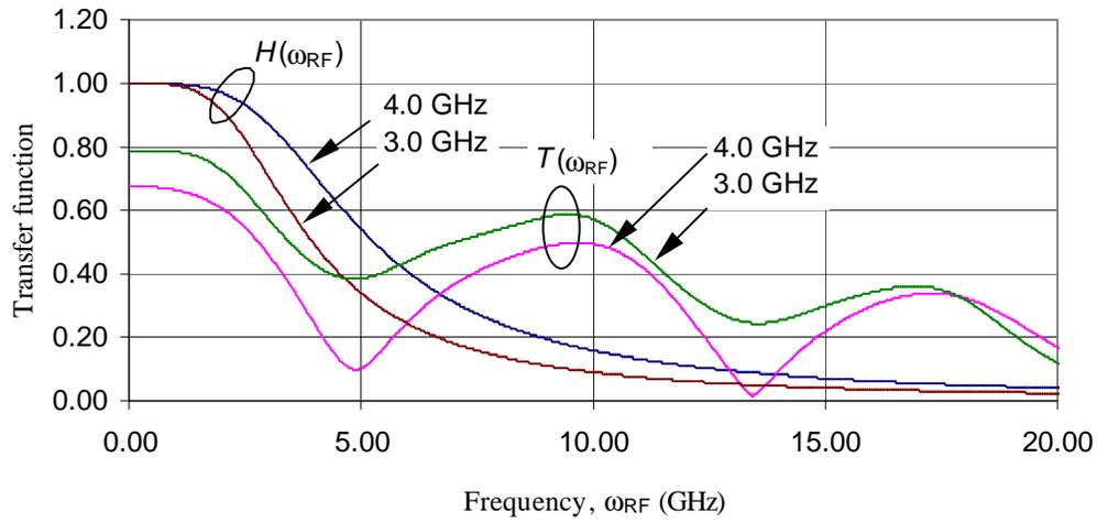
(b) 5-channel system transfer function for 8-pole LPFs
