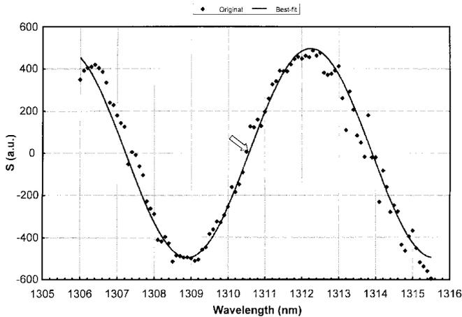
Fig. 3. Wavelength scanning with the target located at  $0^\circ$  and the fixed wavelength  $\lambda_f = 1310.55$  nm. Using a best-fit function to the sine function, the experimentally determined target direction is  $\theta = 0.6^\circ$ .
