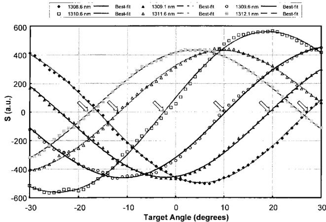
Fig. 2. Target scanning with the receiver pointed to six different “listening” directions, defined by the tunable laser wavelength  $\lambda_t$ . In this demonstration, experimentally determined “listening” directions correspond to the angles where  $S = 0$  and  $S' > 0$ .
