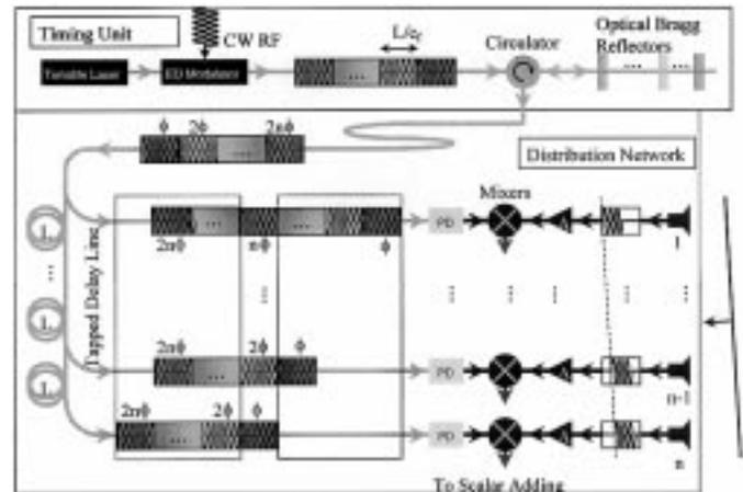
Fig. 1. Basic serially fed receive mode configuration for an array of  $n$  elements. A chirped fiber grating in conjunction with a tunable laser provides the necessary phased delays for virtually continuous directional operation. A second tapped delay line in parallel can be added to achieve almost continuous temporal operation.
