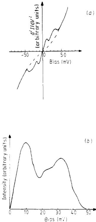
**Figure 1.** (a) The  $d^2I/dV^2$  characteristic of the tunnel junction (full curve) showing the smooth elastic background (broken curve). (b) The  $d^2I/dV^2$  characteristic after subtraction of the elastic background and averaging between positive and negative bias.
