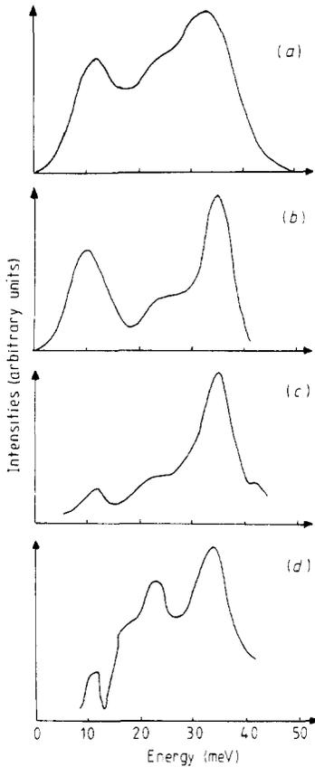
**Figure 5.** (a) The density of states,  $g(\omega)$ , for amorphous germanium (a-Ge) obtained by weighting the  $d^2I/dV^2$  characteristic shown in figure 1(b). (b)  $g(\omega)$  calculated for a network model of a-Ge. (c) Raman spectrum of a thin film of a-Ge. (d) Infrared spectrum of a thin film of a-Ge.
