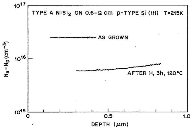
FIG. 1. Hydrogen passivation of boron deduced from *C-V* profiling before and after hydrogenation.
