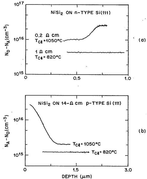
FIG. 4. Presence of *p*-type contaminant revealed by *C-V* profiling for (a) *n*-type and (b) *p*-type substrates after a high-temperature clean ( $T_{cl} \sim 1050^\circ\text{C}$  for 120 sec). For  $T_{cl} \sim 850^\circ\text{C}$  no contamination is detected.
