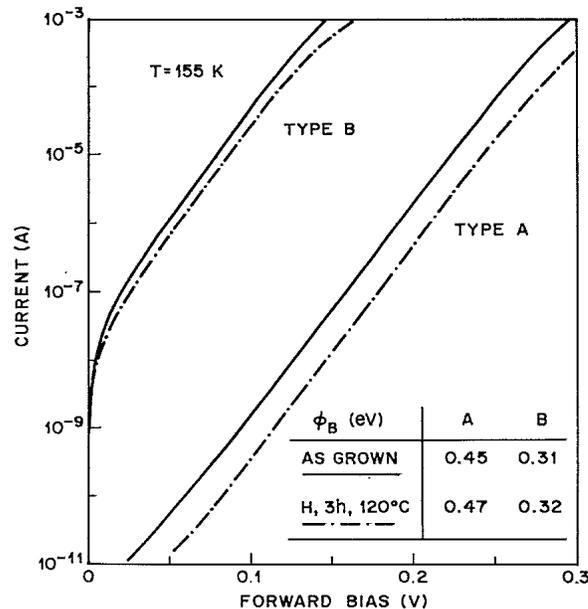
FIG. 2. Typical forward bias *I-V* characteristics before (solid curve) and after (dashed curve) hydrogenation of *A*- and *B*-orientated NiSi<sub>2</sub> on *p*-type Si(111).
