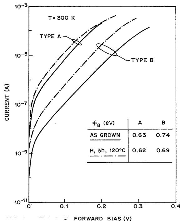
FIG. 3. Typical forward-bias *I-V* characteristics before (solid curve) and after (dashed curve) hydrogenation of *A*- and *B*-orientated NiSi<sub>2</sub> on *n*-type Si(111).
