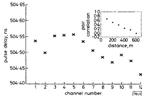
Fig. 2 Pulse delay after transmission through 102m of 12channel ribbon fibre manufactured from high quality graded index MM fibre sequentially cut from the same pull
