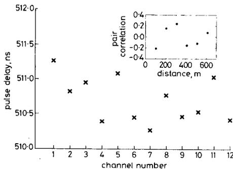
Fig. 1 Measured optical pulse delay after transmission through 103m of conventional 12channel optical ribbon fibre, resulting in maximum interchannel skew of 1005ps
