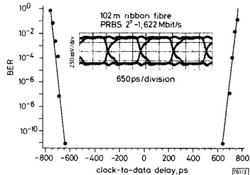
Fig. 3 Eye diagram and BER against clock-to-data delay of parallel synchronous digital transmission over 102m of low skew MM ribbon fibre at 622Mbit/s with 2<sup>7</sup>-1 NRZ PRBS
