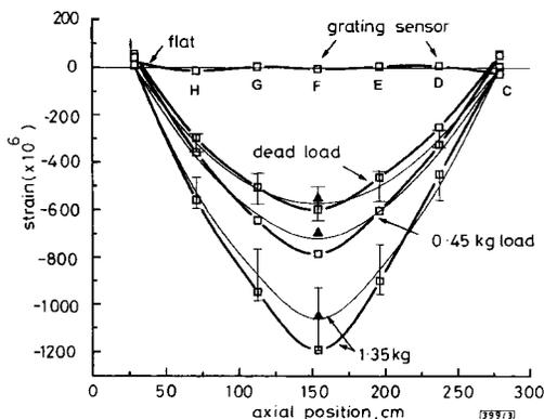
Fig. 3 Comparison of strain in CRTM™ beam measured with FBG sensors and results of finite element and analytical calculations
