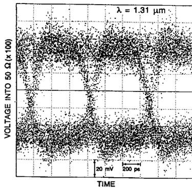
Fig. 8. Detector eye-diagram ( $\times 100$ ) for a 1.5 Gb/s nonreturn-to-zero pseudorandom optical data stream.
