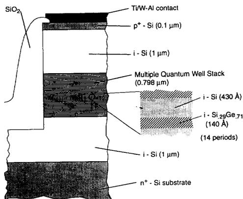
Fig. 3. Layer structure of a pin photodetector.
