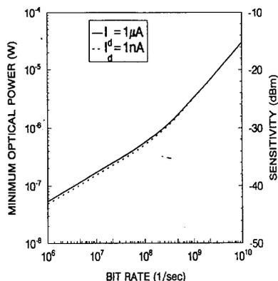
Fig. 10. Calculated sensitivity for a receiver front end consisting of a GeSi pin with  $\eta_{\text{ext}} = 10\%$  and a bipolar transimpedance amplifiers.
