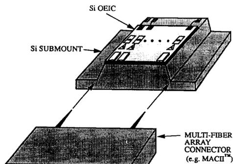
Fig. 11. Diagram of an Si-based integrated receiver mounted on an AT&T MACII<sup>TM</sup> multifiber connector.
