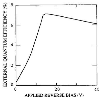
Fig. 6. External quantum efficiency versus applied bias measured for  $\lambda = 1.32 \mu\text{m}$  incident light.
