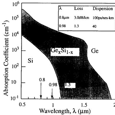
Fig. 1. Absorption coefficients of Ge and Si versus wavelength.
