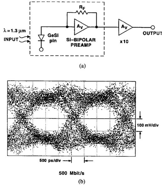
Fig. 7. (a) Block diagram and (b) output eye-diagram at 500 Mb/s for a hybrid silicon-based receiver at  $\lambda = 1.3 \mu\text{m}$ .
