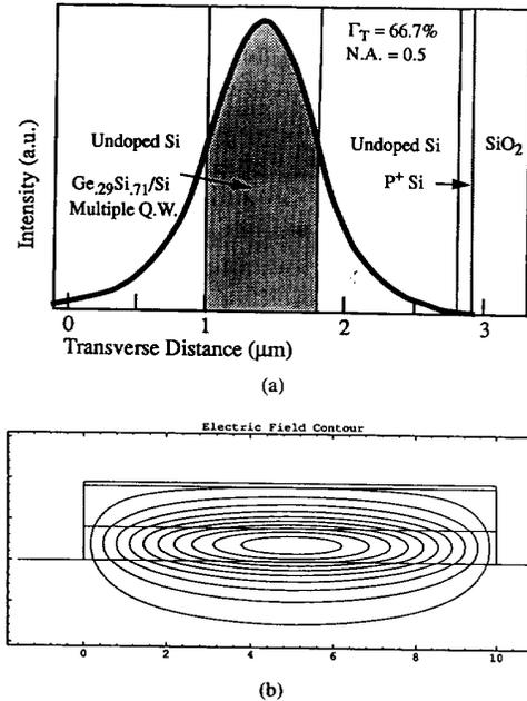
Fig. 9. Calculated (a) transverse and (b) contour plots of optical intensity for the fundamental mode.
