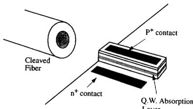
Fig. 2. Schematic of a waveguide pin detector.
