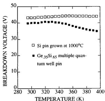
Fig. 5. Temperature dependence of breakdown voltage for GeSi quantum well pin diode shown in Fig. 4 and a device with Si intrinsic layer grown at 1000°C.
