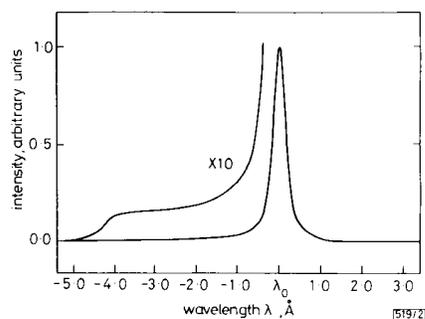
Fig. 2 Experimental time averaged optical spectra observed when  $-0.2 < V_S < 1.5 \text{ V}$  ... 1010 ... bit stream at 1 Gbit/s is applied to absorber section S
