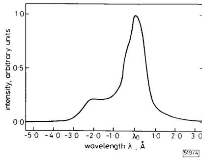
**Fig. 4** Experimental time averaged spectrum for conventionally modulated DFB laser
