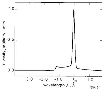
**Fig. 5** Calculated time averaged spectrum of conventionally current (directly) modulated laser
