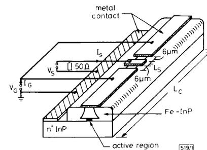
Fig. 1 Schematic diagram of intracavity loss modulated DFB laser
