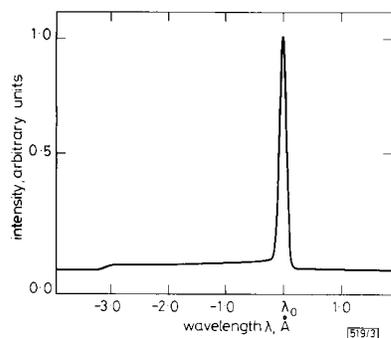
Fig. 3 Calculated time averaged spectrum of intracavity loss modulated laser
