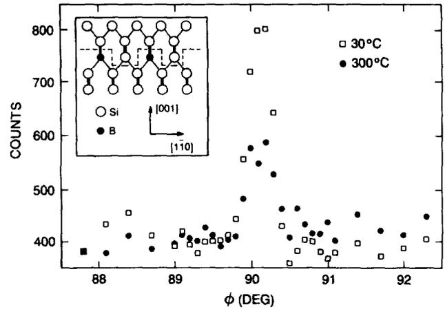
FIG. 6. Comparison of grazing incidence x-ray diffraction azimuthal scans through the (3/2,0) diffraction spot for Si(100)-(2 $\times$ 1) boron buried structures capped by growth at room temperature, and at  $\approx 300^\circ\text{C}$ . The boron coverage was 1/2 monolayer in both cases and the silicon growth rate was 0.1 Å/s. The inset shows a proposed model of the (2 $\times$ 1) structure.
