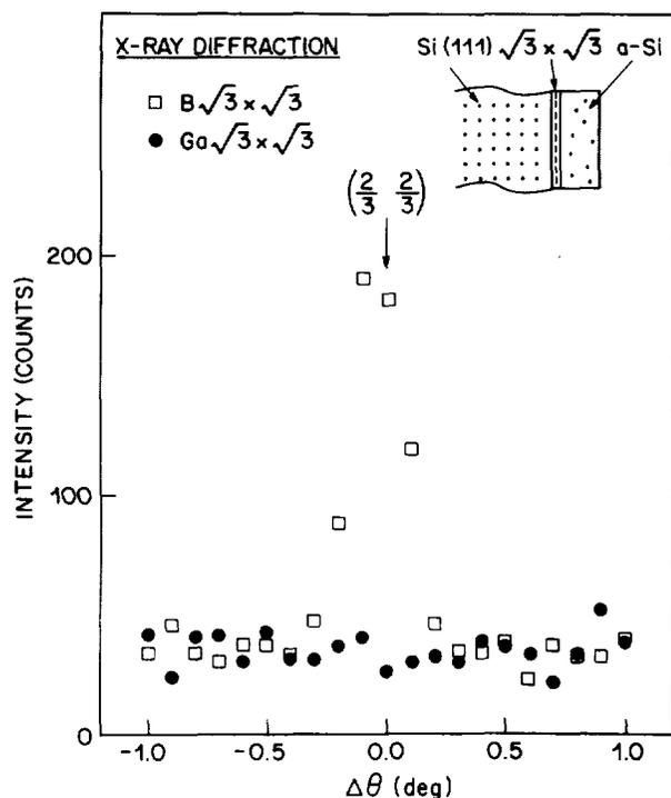
FIG. 2. Rocking scan through the  $(2/3, 2/3)$  surface x-ray diffraction rod for buried boron and gallium surface structures on Si(111). The intensity units refer to reflectivity in counts per constant integrated incident beam flux.
