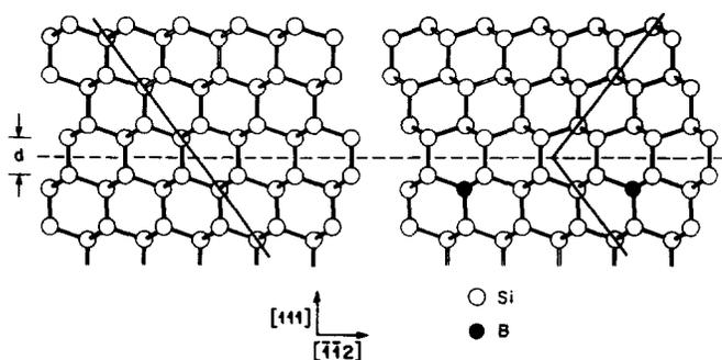
FIG. 3. Ball and stick models for the film orientation and interface structure for 0- (left) and 0.33-ML (right) boron coverages. The  $\sqrt{3} \times \sqrt{3}$  reconstruction of the interface is introduced because boron occupies substitutional sites, occupying every third site in a single monolayer at the interface.
