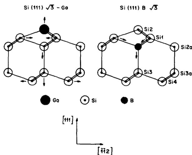
FIG. 1. Model of the Si(111)- $\sqrt{3}$ Ga structure and proposed structure for Si(111):B $\sqrt{3}$  (right). Arrows indicate the direction of displacements from the ideal tetrahedrally bonded configuration.
