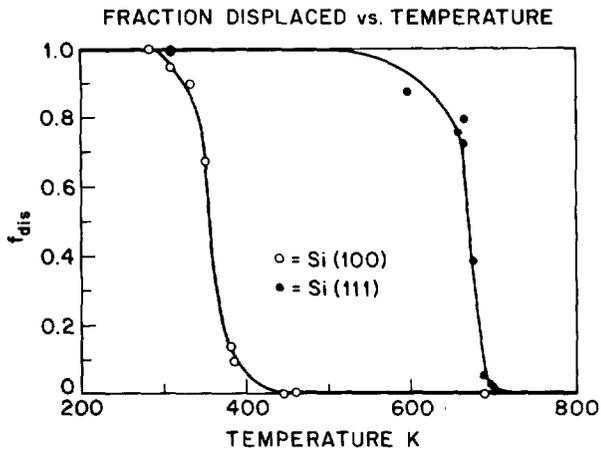
FIG. 5. Ion channeling yield vs growth temperature of thin silicon films on Si(100) and Si(111).
