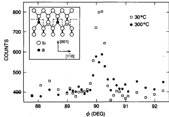
Fig. 6. Comparison of grazing incidence X-ray diffraction azimuthal scans through the  $(\frac{3}{2}0)$  diffraction spot for Si(100)-(2  $\times$  1) boron buried structures capped by growth at room temperature, and at  $\approx 300$  °C. The boron coverage was 1/2 monolayer in both cases and the silicon growth rate was 0.1 Å/s. The inset shows a proposed model of the (2  $\times$  1) structure.
