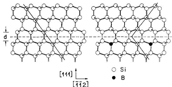
Fig. 4. Ball and stick models for the film orientation and interface structure for 0 (left) and 0.33 ML (right) boron coverages. The  $\sqrt{3} \times \sqrt{3}$  reconstruction of the interface is introduced because boron occupies substitutional sites, occupying every third site in a single monolayer at the interface.
