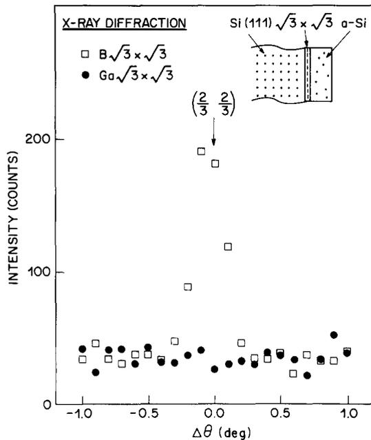
Fig. 2. Rocking scan through the  $(\frac{2}{3}, \frac{2}{3})$  surface X-ray diffraction rod for buried boron and gallium surface structures on Si(111).
