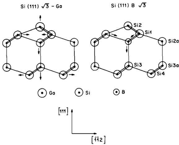
Fig. 1. Model of the Si(111)-Ga- $\sqrt{3}$  structure and proposed structure for Si(111)-B- $\sqrt{3}$  (right). Arrows indicate the direction of displacements from the ideal tetrahedrally bonded configuration.
