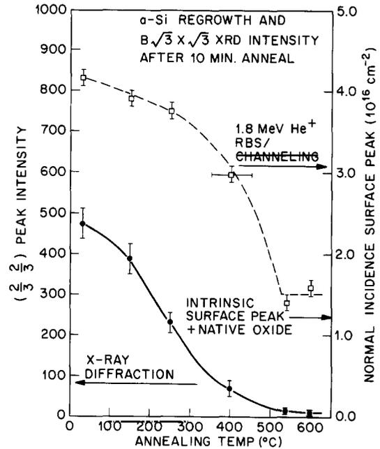
Fig. 3. Dependence of the  $(\frac{2}{3}, \frac{2}{3})$  surface X-ray diffraction integrated intensity as a function of annealing temperature for the boron  $\sqrt{3} \times \sqrt{3}$  surface structure originally covered with a-Si ( $\sim 100 \text{ \AA}$ ) (filled circles). Also shown is the temperature dependence of normal incidence channeling for the Si overlayer indicating complete epitaxial regrowth at  $\sim 500^\circ \text{C}$ .
