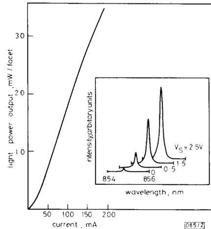
**Fig. 2** Light intensity per facet against pulsed gain current
