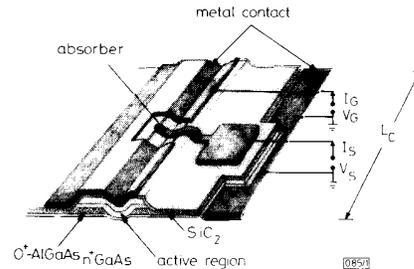
**Fig. 1** GRINSCH single quantum well laser diode
