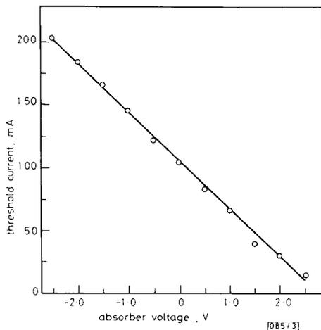
Fig. 3 Laser threshold current against absorber voltage
